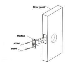
Place the latch through the latch hole positioned correctly for latching your door. Leave the latch loose until both the front lock body and back iron panel are installed.
