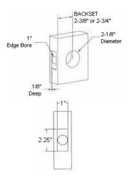
If you are installing the eRL-08 Lock Device in a door with pre-drilled holes, the lock will fit most standard doors. To confirm that the lock will fit your door, please verify the following measurements:
